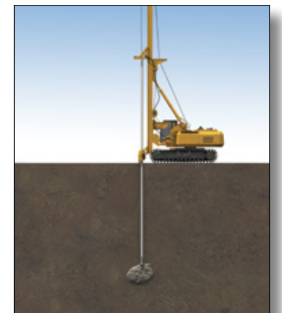
Boulders may even lead to a total failure to drill down to desired depth
